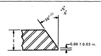
$^{(1)}$  Or 1 in. at option of the manufacturer. (2) Fittings NPS 24 and smaller may be furnished with 37 1/2°  $^\pm$  2 1/2° bevel at option of the manufacturer.
