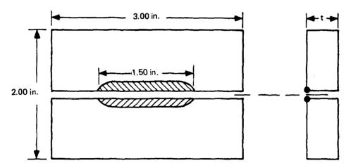
Longitudinal-Bead Underbead Cracking Test Specimen Figure X2-1
