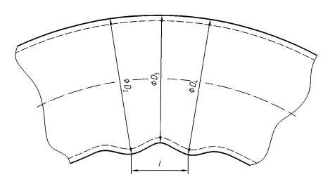
Figure 3 — Schematic diagram for measurement of waving
